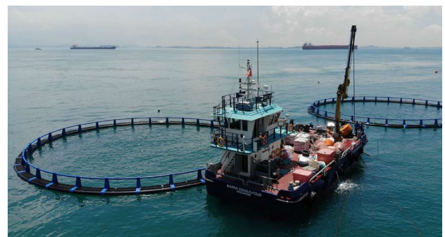
Barra Endeavour was used to deploy the new farm anchors and mooring system, cages and nets. Harvesting and fish transfers are also part of its designed capabilities.
